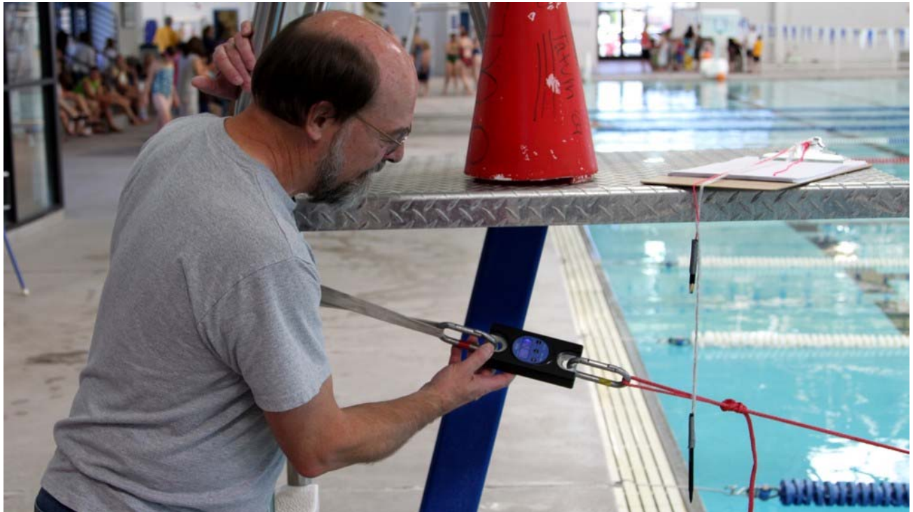
Dr. Hanlon checks the load cell as the underwater test stand is assembled and aligned. A surrogate scooter was used to ensure that the apparatus was configured correctly, then thrust testing began.
