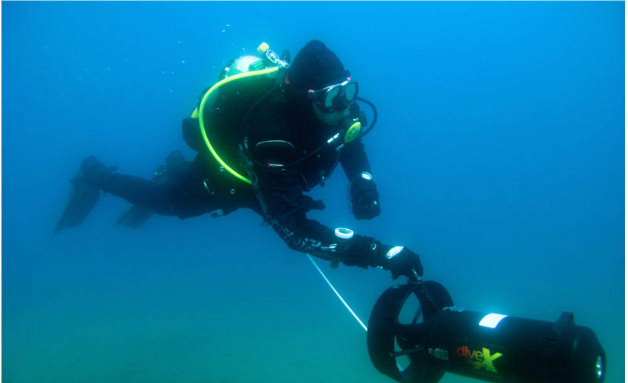
Running by the clock: Stopwatch in hand, test diver Vic Erickson begins calibrating a scooter for the cruise speed test. Photo by Chuck Weber
